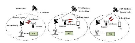
The attacker tries to cause interference to the feeder link from the NTN payload to the NTN-GW.
